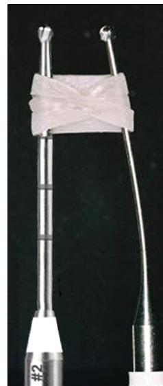
Fig. 5: Stiffness of Munce Bur shaft v. noodling of Mueller Bur.
